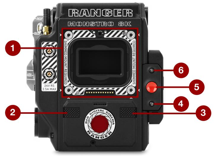
Figure: Camera Body Controls and Features
