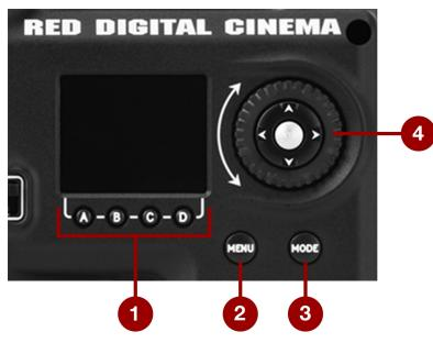
Figure: Side LCD and Navigation
