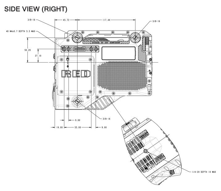
Figure: Camera Side View (Right)
