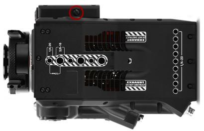
Figure: Focus Hook Screw Storage Location
