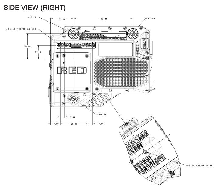
Figure: Camera Side View (Right)
