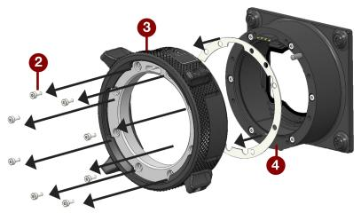
Figure: Shim Installation
